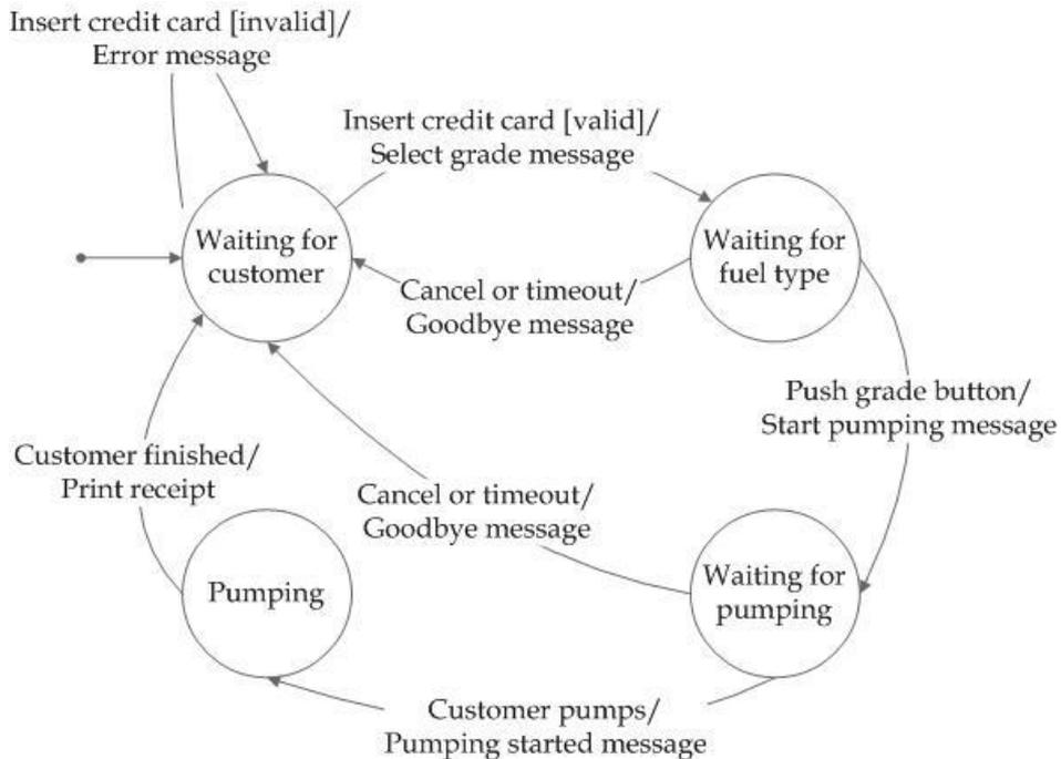
Assume that you want to develop the minimum number of tests to cover each transition in the state transition diagram. Assume further that each test must start at the beginning state, waiting for customer, and each test ends when a transition arrives at the beginning state. How many tests do you need?
